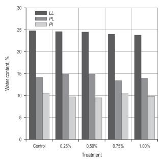
**Fig. 2** Effect of different percent of CBR PLUS on Atterberg limits including Plastic Index (*PI*), Plastic Limit (*PL*) and Liquid Limit (*LL*)
