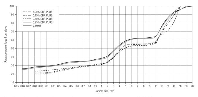
Fig. 4 Curve of weight distribution of particle size for materials treated by different percentages of CBR PLUS
