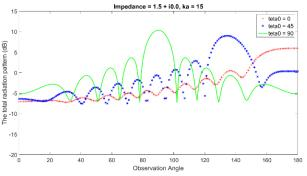
**Figure 6.15.** The total radiation pattern for *ka*=15
