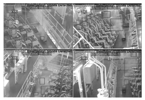
*Figure 8: Video smoke detection using 4 different angle cameras in a 3 sec time gap Source: author*
