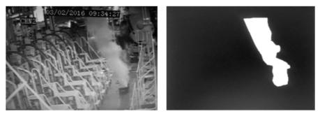
Figure 6: Isolation of detected smoke Source: author
