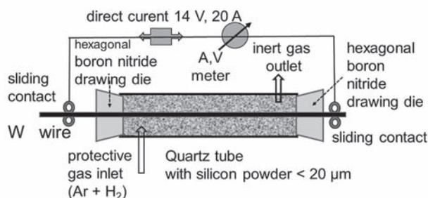
**Figure 2** Scheme of  $WSi_2$  coatings preparation on a tungsten wires
