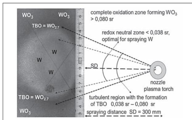
**Figure 4** Evaluation scheme of footprint deposition tungsten by thermal spraying
