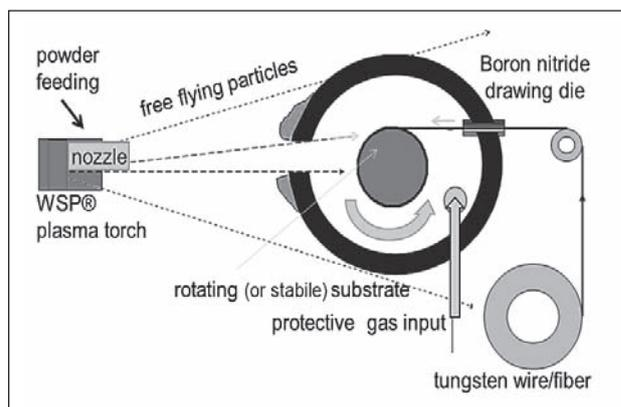
**Figure 7** Scheme deposition on the moving parts of tungsten substrates
