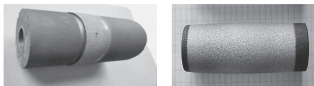
**Figure 8** Examples of W-coated parts on graphite
