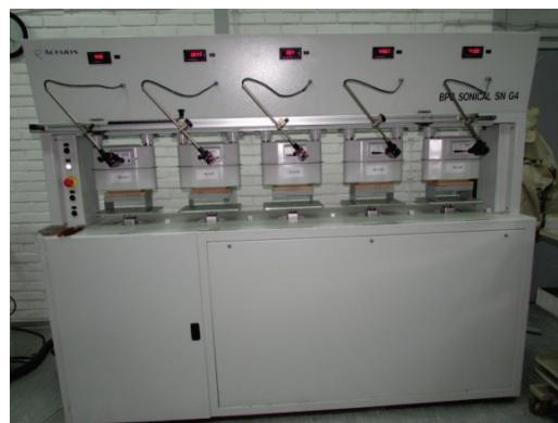
Figure 1 Testing rig BPG-R SONICAL SN G4 [4]
