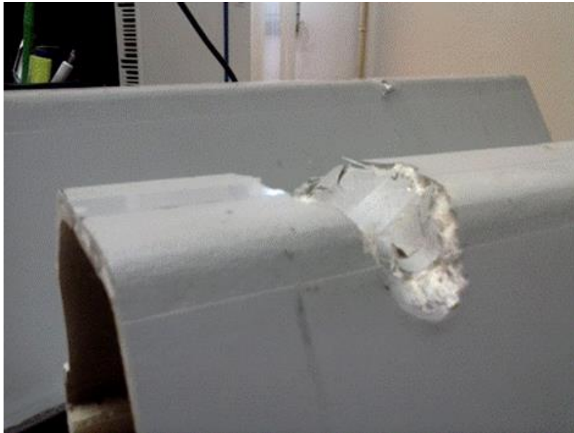
Figure 2 Local beam deformation [4]
