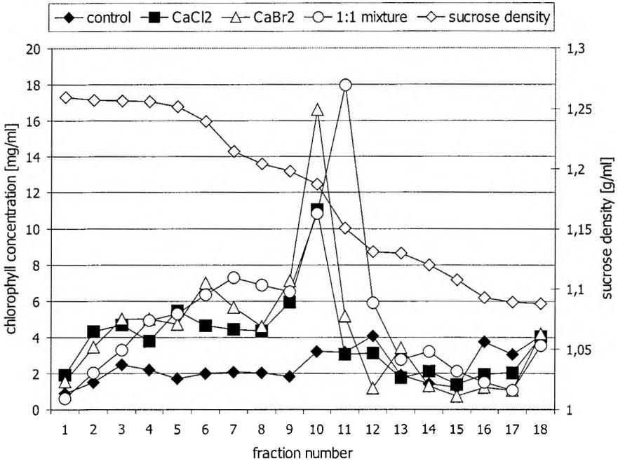
**Fig. 2.** Sedimentation profiles of chloroplasts (determined as chlorophyll content) from duckweed *Lemna minor* L. cultivated on control medium as well as on media containing CaCl<sub>2</sub>, CaBr<sub>2</sub> and their 1:1 mixture.
