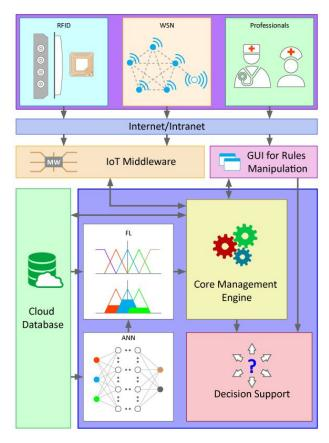
Figure 2. System architecture of IoT-HAMS
