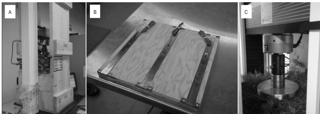
Fig. 1 A) Load frame with custom built load test structure, B) Three strain gauges installed below steel channels (channels were turned upside down to show strain gauges), C) Horizontal crosshead of load frame with load cell and steel circular loading disk resting on a softwood brush mat
