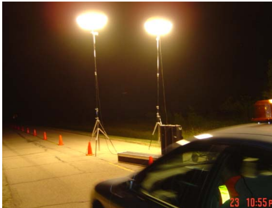
Figure 4.36. Two balloon lights arrangement.
