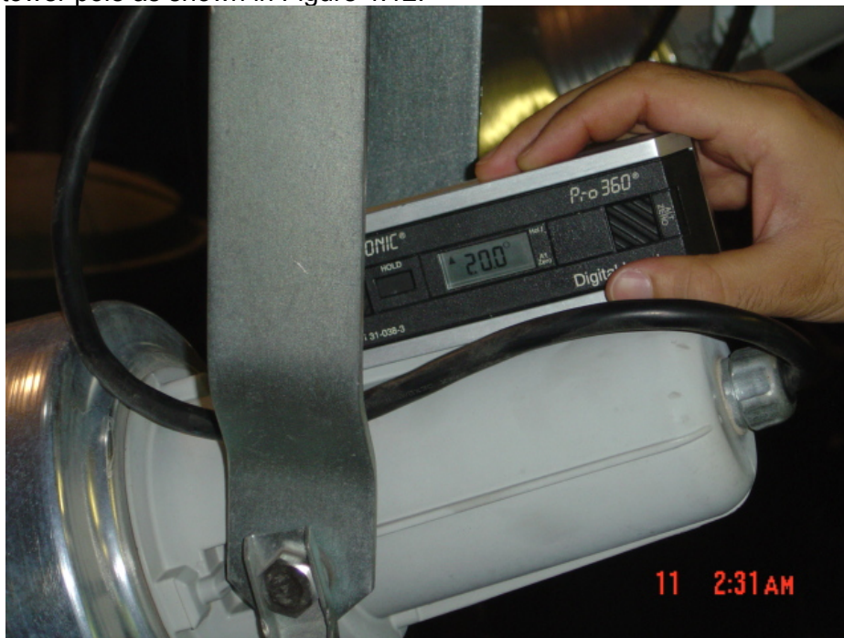
Figure 4.11. Angle locator used to measure aiming angles.
