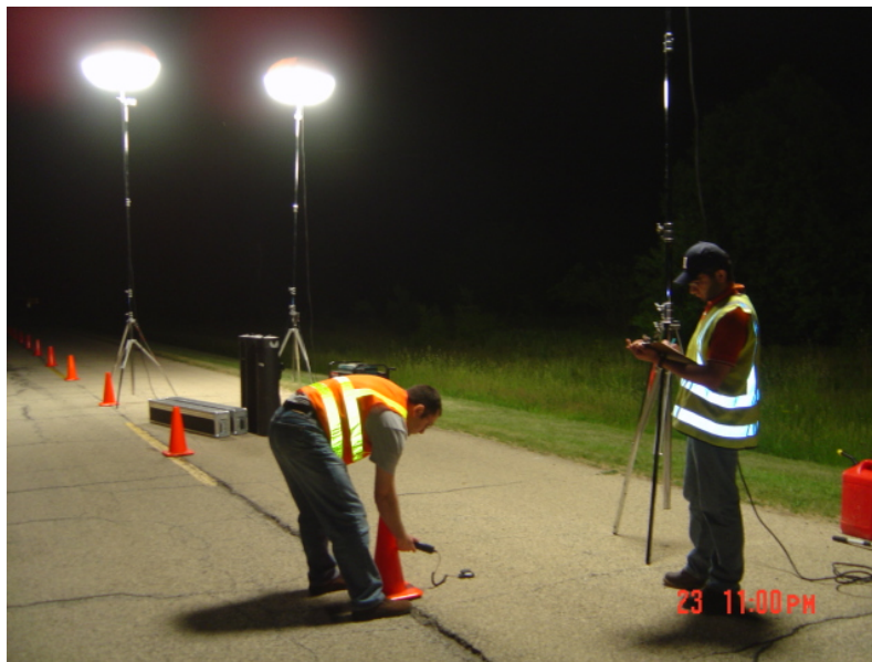
Figure 4.20. Horizontal illuminance measurements.
