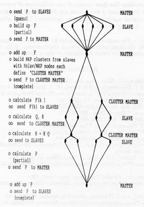
Figure 7. Communication structure of the SCF program, including parallelization of the matrix diagonalization.
