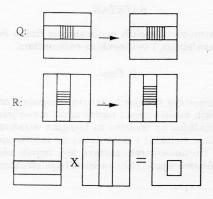
Figure 8. Parallelization of the QR-algorithm. Calculation of matrices Q (distributed by rows) and R (distributed by columns) and matrix multiplication RQ.
