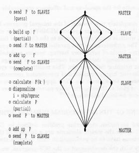
Figure 6. Parallel concept of the SCF program without performing diagonalization in parallel.
