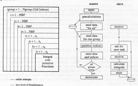
Figure 1. Loop-structure of the crystal orbital two electron integral program.
