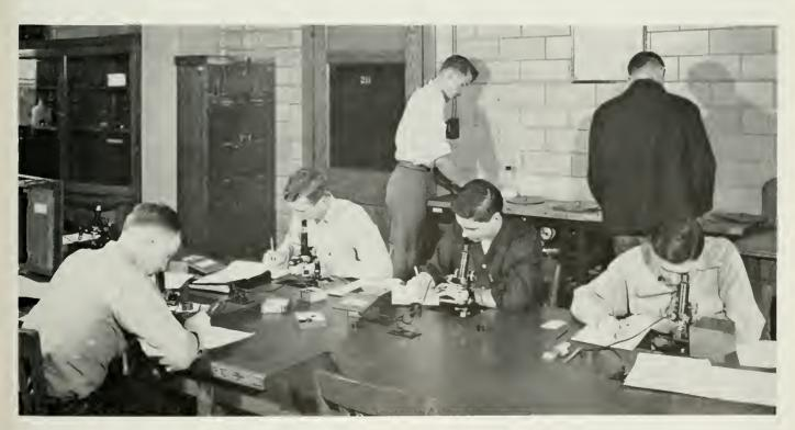
Students in Metallurgical Engineering are required to take several laboratory courses. Several students are shown doing metallographic work in one of the metallurgical laboratories.
