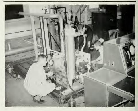
Figure 1. As part of the practical application of the theory taught in the clossroom, several Mechanical and Industrial engineering students are shown running tests on the adiabatic compression machine in the Internal Combustion Engine Laboratory.
