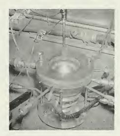
Figure 1. The thermal electric rocket motor produces a plasma consisting of an electrically neutral conglomeration of ions, electrons and neutral atoms with temperatures up to 30,000 degrees F.
