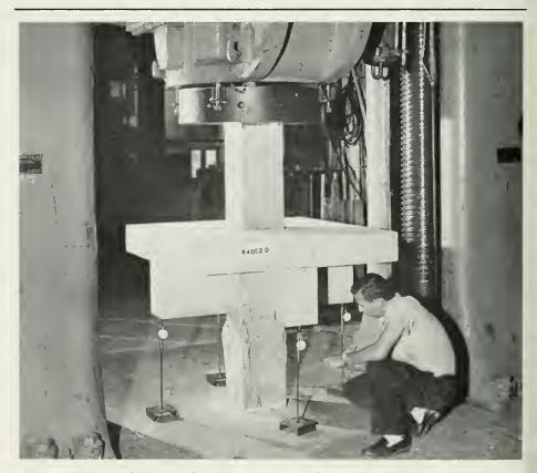
Figure 1. A groduate student is examining the failure in a reinforced concrete specimen. The specimen was loaded by the partly visible machine, which can exert 3,000,000 pounds of compression or expansion.
