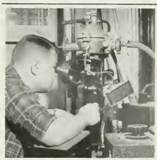
Figure 2. High temperature microscope used in Ceramic Engineering Department to study changes in microstructure of moterials during heating to high temperatures.
