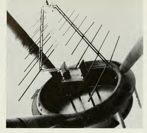
Figure 1. Pictured above is a Log-Periodic Dipole Antenna. This type antenna was invented and developed at the University of Illinois.
