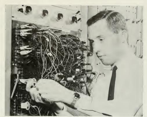
Richard E. Covert, Iowa State BSME '62, utilizes an analog computer to study heat transfer transients and their effect on the control mechanism of a mobile military compact reactor being developed by the Allison Division of General Motors under contract to the Atomic Energy Commission. Covert is one of several young engineers now engaged in various studies connected with nuclear powerplant engineering programs at Allison.
