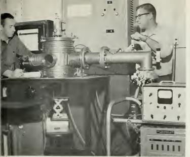
Figure 1. Research staff in the Ceramic Engineering High Temperature Technology laboratory assemble an inductionheated cell used for thermal conductivity, oblation transpiration and diffusion studies of aerospace materials to as high as 5000 degrees F.
