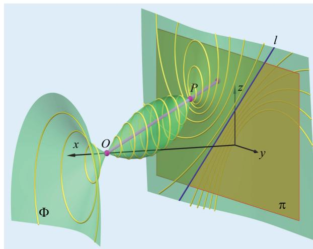
Figure 6: The quartic surface  $\Phi$  with its circles in planes parallel to  $\pi$  has a singularity at  $O$  and  $P$ .  $\Phi$  intersects  $\pi$  in the line  $l$  and the ideal line  $p_2$  of  $\pi$ , the latter with multiplicity three.
