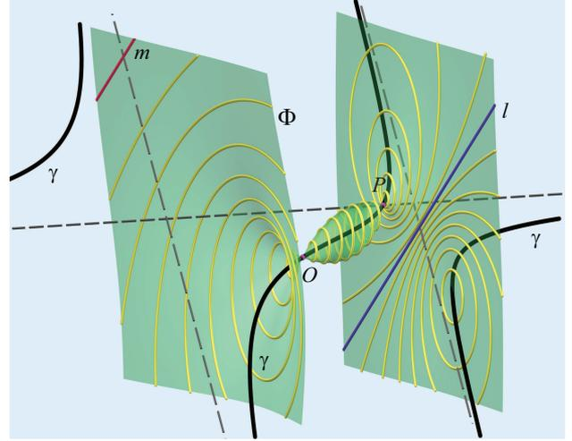
Figure 8: The cubic curve  $\gamma$  carries the centers of all circles on  $\Phi$ . Its ideal doublepoint  $(0 : 0 : \eta : \zeta)$  is the ideal point of the lines orthogonal to  $l \parallel m$ . The tangent of  $c$  at the third ideal point  $(0 : 1 : 0 : 0)$  passes through  $P$ . The three dashed lines are  $\gamma$ 's asymptotes.
