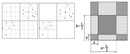
Figure 2: Dissection of a bounding box, a quadtree, and a shifted quadtree
