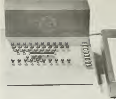
Figure 1. Students "type" their responses on a keyset to communicate with the central computer. A newer keyset will be in operation soon.
