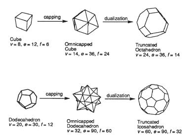
Figure 4. Applications of the leapfrog transformation to the cube and the regular dodecahedron.
