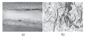
Figure 3 Presentation of the corrosion phenomenon of the material in the welded constructions a - general view of the areas subjected to corrosion, b- corrosion cracking in the structure of the material
