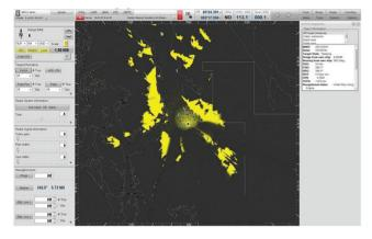
3. b. Radar receiver in saturation in the 160° sector 4 3. b. Radarski prijamnik u zasićenju kod 160° sektor 4
