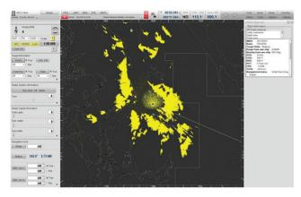
3. a. Radar display without the impact of intentional interferences 9
