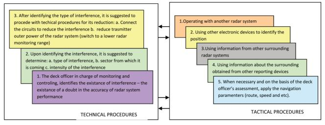
Figure 1. Procedures of the radar system operator in case of intentional jamming 4 Slika 1. Postupci operatora radarskog sustava u slučaju namjernog ometanja 4
