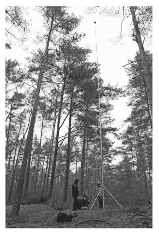
**Fig. 1** An aluminum telescopic mast with the GNSS receiver in the Gluchów forest district (photo: Dariusz Górscy)
