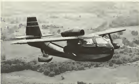
Figure 27—Amphibian airplane with a hull for water landings and wheels (retractable) for runway landings.
