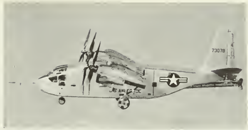
Figure 39—X-18 IN FLIGHT TESTS—Shown is the 16½ ton X-18 during flight tests over Edwards Air Force Base, Calif. Wings have reached an angle of attack of 50 degrees during flight. Now in a ground program to study the effects of downwash during simulated hovering, the X-18 is expected to be back in flight tests at a later date far full hovering and vertical operation.
