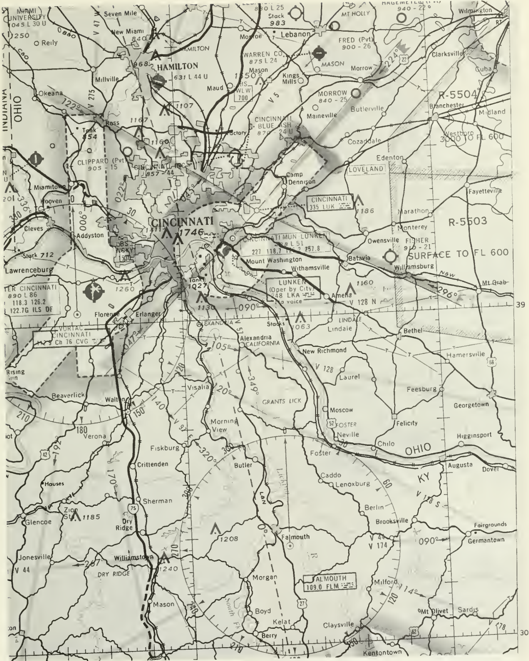
Figure 107—Part of a Sectional Chart Showing Four Directional Beams Transmitted by a Low Frequency Station
