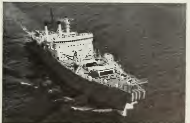
C. S. LONG LINES lays and maintains Bell System undersea telephone cables that provide dependable overseas transmission.
