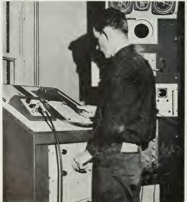
John Kimball, a junior in engineering physics and a student technician in the antenna laboratory, operates the polar pattern-recorder in the low-frequency antenna testing range.
