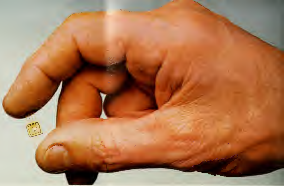
This tiny device is an ultra-reliable Westinghouse TV amplifier
