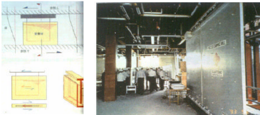
Figure 2.51. Wall viscous dampers: dissipative mechanism ( left ) and lab test ( right ).
