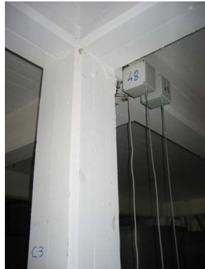
(a) Col. 3 after 0.15g PGA test
