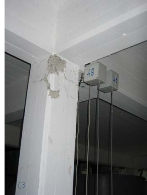
(b) Col. 3 after 0.20g PGA test
