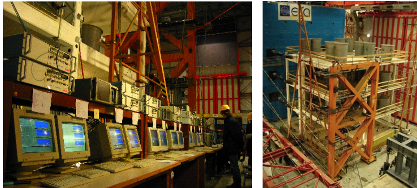
Figure 7.2 Setup for the pseudo-dynamic testing
