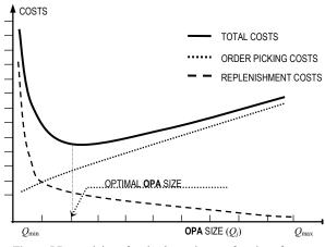
Figure 5 Determining of optimal opa size as a function of costs
