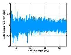
Fig. 4. Benefit of multipath correction: The strong multipath pattern is removed, and thus the code residual contains a nearly white Gaussian noise
