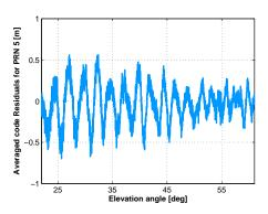
*Fig. 3. The multipath estimate of the link between station Günzburg and PRN* 5
