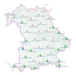
Fig. 1. The SAPOS network in Bavaria. Green triangles indicate the stations where the observations were taken. The station Günzburg in blue triangle shows strong repeatable multipath error.
