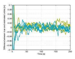
Fig. 8. The estimation error of orbit corrections, i.e. light green curves indicate the in-track errors, and blue curves the cross-track errors
