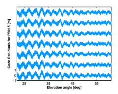
Fig. 2. The code residuals observed at station Günzburg for PRN 5 between the observed period over a week. To distinct among others, the curves have been shifted artificially.
