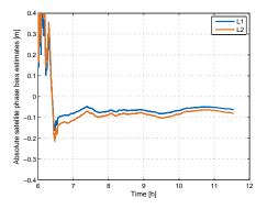
Fig. 7. Absolute satellite phase bias estimates of PRN 24 on both frequencies, which has shown a high stability over the total visible period
