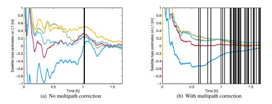
Fig. 5. Satellite bias estimation without and with multipath correction. The multipath error propagates into the phase bias estimates which show large variations over time. The corrections remove the oscillations on the phase bias estimates and thus enable more stable bias estimates. The integer ambiguity fixing benefits from the corrections, where a much earlier fixing and much more fixings (40 out of 90 instead of 2) are enabled.
