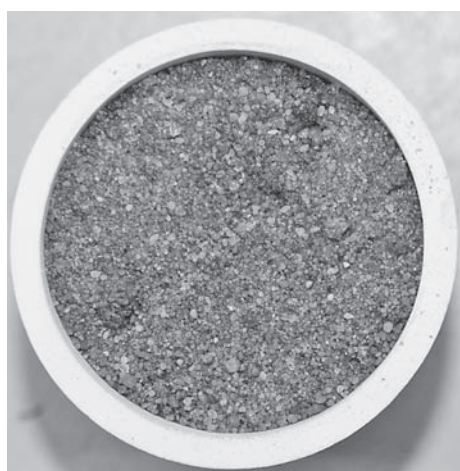
Figure 7 View of waste moulds and cores before utilization in the microwave chamber; moulding sand M4
