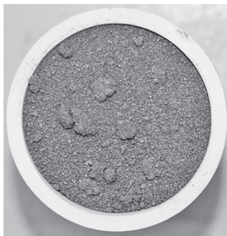
Figure 4 View of waste moulds and cores before utilization in the microwave chamber; moulding sand M1
