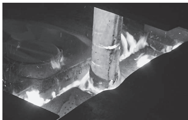
Figure 1 Plates of formed mould prepared by means of manual compacting during industrial tests of powder application in concast mould
