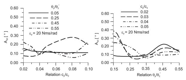
Fig. 6 Diagram of twist angles of the torsional vibration amplitudes  $(A_{6/1})$  at the engine pulley  $(\theta_1)$  depending on the relative stiffness and relative moment of inertia of the inertial mass of the balance weight damper
