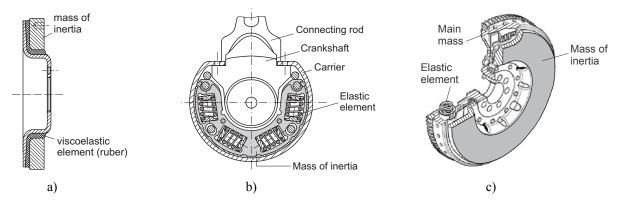
Fig. 1 Three different TVDs for road vehicles IC engines
