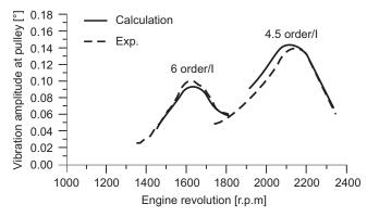
Fig. 5 Diagram of calculated and experimentally obtained twist angles of the torsional vibration amplitudes at the pulley for the engine with an elastic TVD
