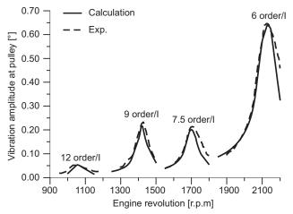
Fig. 4 Diagram of calculated and experimentally obtained twist angles of the torsional vibration amplitudes at the pulley for the engine without a TVD
