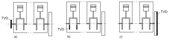
Fig. 2 TVD mounting places in IC engines
