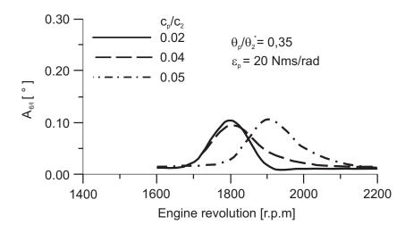
Fig. 7 Diagram of twist angles of the torsional vibration amplitudes  $(A_{6/l})$  at the motor pulley  $(\theta_l)$
