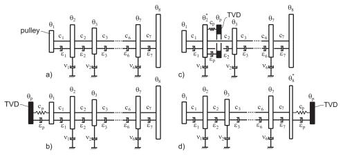
Fig. 3 Physical models of torsional vibration systems with different dampers
