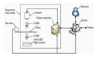
Fig. 9. Float glass inspection system [19]
