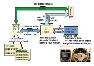
Fig. 10. System configuration for validation testing of vehicle instrument cluster [20]
