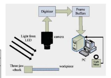
Fig. 2. A typical vision system operation [2]
