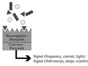
**Figure 1.** Mode of operation of a biosensor **Slika 1.** Princip rada biosenzora
