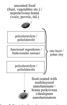
Figure 5. Principle of nanolaminates creation Slika 5. Princip nanošenja nanolaminata
