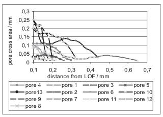
Figure 7 Size of pores inside a welded joint
