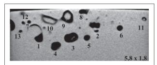
**Figure 4** Dimensional analysis of porosity area (pores are numbered from 1 to 13)
