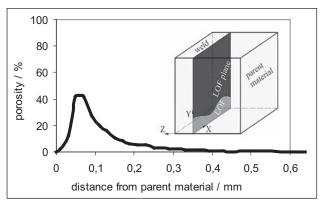
Figure 5 Change in porosity as per weld section
