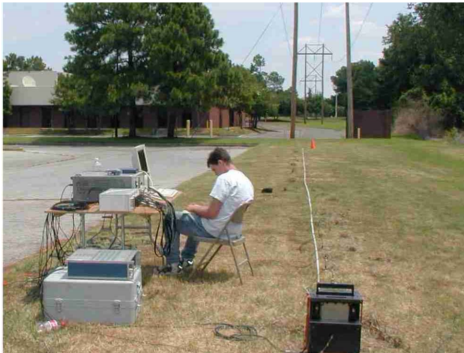
Figure 4.4 Picture of Active f-k Testing Performed in Memphis, TN.
