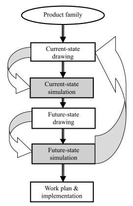
Figure 3 Steps of new production reorganization tool Slika 3. Koraci novog alata za reorganizaciju proizvodnje
