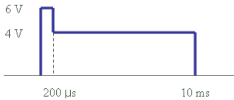
Figure 5.13 : A typical analog guide signal for the guiding lasers
