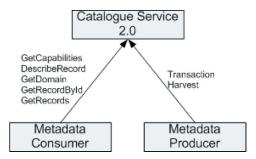
Fig. 4. CSW conceptual architecture.
