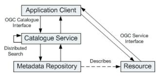
Fig. 2. Reference model architecture.
