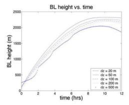
**Figure 1**. BL height evolution as estimated by the TM model, at different vertical resolutions (dz); the surface heat flux H<sub>0</sub> varies according to  $H_0 = H_{max} \sin \omega t$  (here  $2\pi\omega^{-1} = 24 h$ ,  $H_{max} = 0.2 \text{ K m s}^{-1}$ ).
