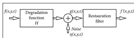
Figure 1. A model of the image degradation and restoration process
