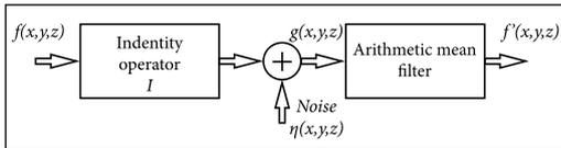
Figure 4. A model of the image degradation with identity operator as the degradation function, and arithmetic mean filter as the restoration filter
