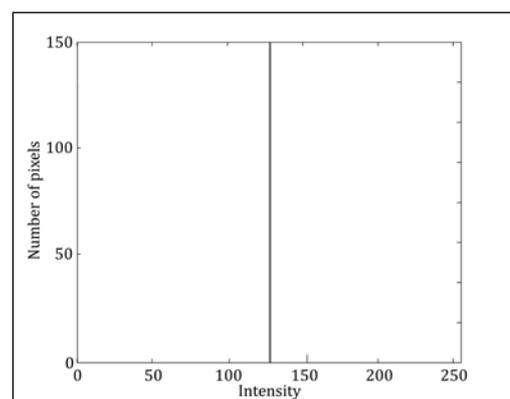
Figure 2. The histogram of a reproduced unit impulse in process without degradation
