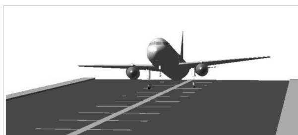
Figure 6. The animation sequence of landing airplane with present lateral wind - one gear landing case.
