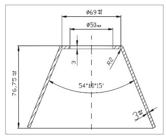
Figure 1. The insert diagram
