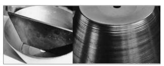
Figure 8a, b. Checking the insert height, draw piece with furrows on the surface
