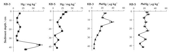
Figure 4 Depth distributions of total mercury and methylmercury in sediments from the Kaštela Bay, collected near chlorine-alkali plant (KB-3 and KB-5 cores were sampled at the same location, KB-3 in February 2001 and KB-5 in October 2001)
