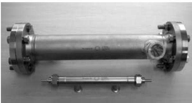
Fig. 5 – Photographs of a single tube and a seven tube Pervatech module
