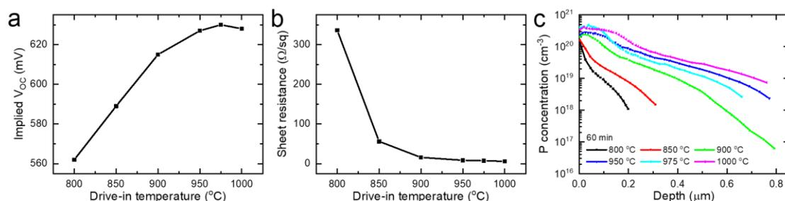
Figure 5.1 The dependences of (a)  $iV_{\text{OC}}$ , (b)  $R_{\text{sh}}$ , and (c) doping profile on drive-in temperature for n-type wafer doped by P spin-on doping.
