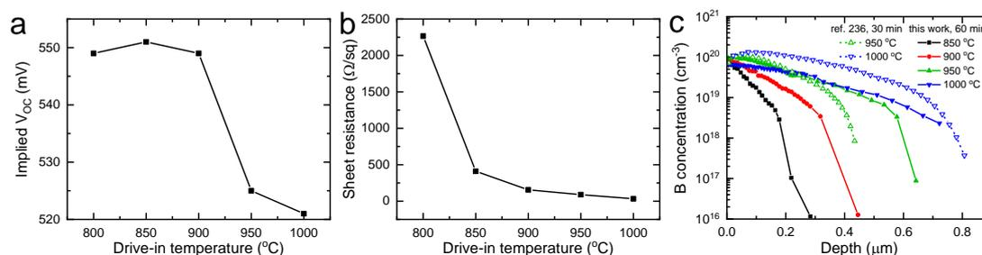
Figure 6.1 The impacts of drive-in temperature on (a) implied open-circuit voltage, (b) sheet resistance, and (c) doping profile for B spin-on doping on n-type wafers.
