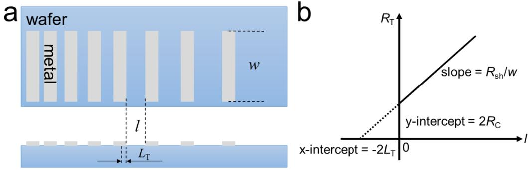
Figure 4.4 (a) The distribution of fingers on wafer surface and (b) typical plot for TLM measurement [196, 216]. Figure 4.4 shows the typical structure of the sample for TLM method. A set of rectangle metal fingers are formed on the single side surface. The dimension of these fingers is same, where  $w$  is the width. But the interval ( $l$ ) between two rectangle metal contacts varies. The measured total resistance ( $R_t$ ) is given by equation 4.6:
