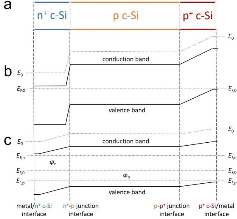
Figure 1.1 (a) Simple schematic of a n<sup>+</sup>-p-p<sup>+</sup> silicon solar cell structure; its band diagram in (b) dark and equilibrium condition and in (c) illuminated and quasi-steady state [3, 11].
