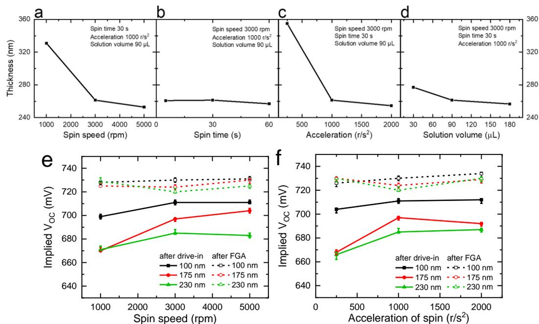
Figure 5.2 The phosphorus-containing SOG thickness as a function of (a) spin speed, (b) spin time, (c) spin acceleration, and (d) solution volume;  $iV_{OC}$  values of samples for poly-Si thicknesses of 100 nm (black), 175 nm (red) and 230 nm (green) coated by (e) various spin speeds and (f) spin accelerations, after annealing at 975 °C for 60 min (filled symbols, solid lines) and after FGA (open symbols, dashed lines).
