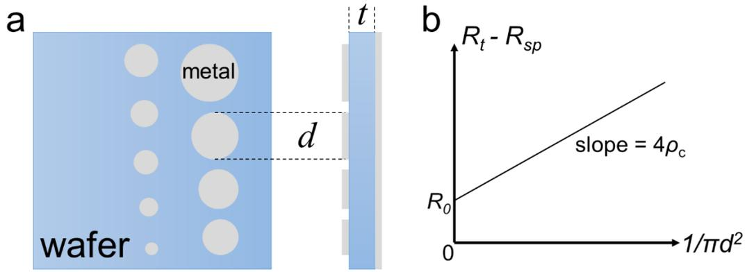
Figure 4.3 (a) The sketch of sample structure and (b) typical plot of Cox-Strack measurement [195, 216].
