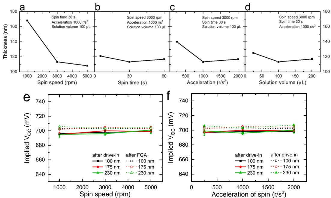
Figure 6.2 The correlation of boron-containing SOG thickness with (a) spin speed, (b) spin time, (c) spin acceleration, and (d) solution volume; the impacts of (e) spin speed and (f) spin acceleration on  $iV_{OC}$  values for 100 nm (black), 175 nm (red) and 230 nm (green) poly-Si, after 950 °C-60 min drive-in process (filled symbols, solid lines) and FGA process (open symbols, dashed lines).
