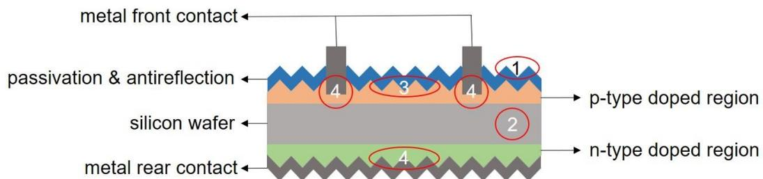
Figure 1.3 Sketch of the structure of a typical diffused silicon solar cell. Region 1 is front layer. Region 2 is wafer bulk. Region 3 is wafer/front layer interface. Region 4 is wafer/contact interface.
