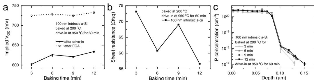
Figure 5.4 The (a)  $iV_{OC}$  values (before and after FGA), (b)  $R_{sh}$ , and (c) doping profiles for 100 nm deposited Si samples for various hard baking time.
