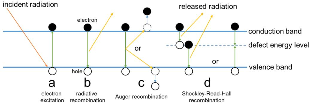
Figure 1.4 Sketches of carrier behaviours in silicon wafer bulk: (a) electron excitation, (b) radiative recombination, (c) Auger recombination, and (d) SRH recombination [30, 31].
