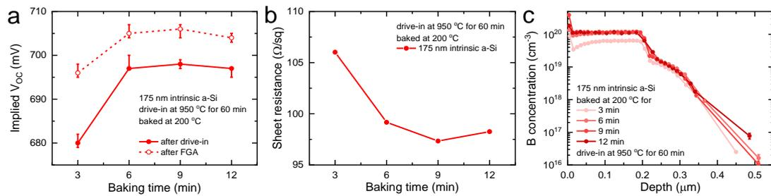
Figure 6.4 The dependence of (a)  $iV_{OC}$  before and after FGA, (b) sheet resistance, and (c) doping profiles on various hard baking dwell times for 175 nm poly-Si samples for B spin-on doping.
