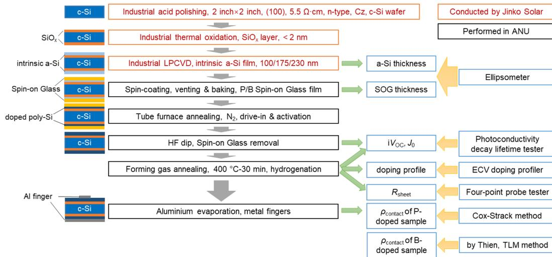
Figure 4.1 The sample structure schemes, process flow, and measurements in this research.
