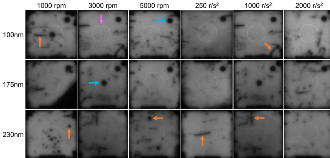
Figure 5.3 The PL images of n-type poly-Si passivating contact samples coated using various spin speeds and different spin accelerations. The poly-Si thickness included 100, 175, and 230 nm. The exposure time was 0.5 s, and illumination intensity was 0.875 suns for all samples.
