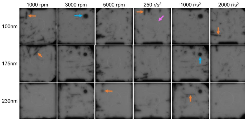
Figure 6.3 The PL images of p-type poly-Si passivating contact samples coated with various spin speeds and different spin accelerations. The left 100, 175, and 230 nm indicate the poly-Si thickness. The exposure time was 0.5 s, and illumination intensity was 0.875 suns for all the samples.
