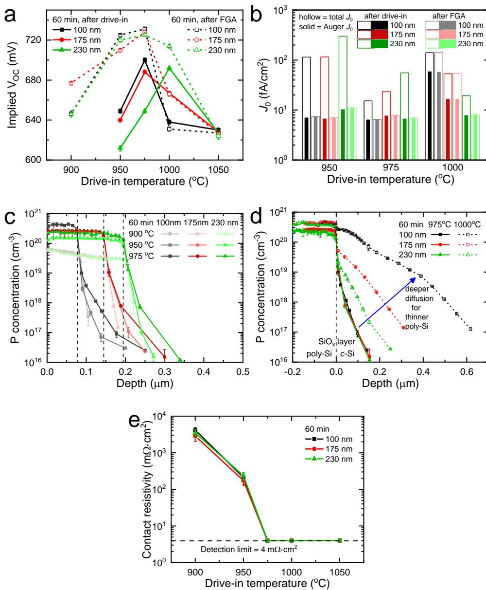
Figure 5.5 (a)  $iV_{OC}$  values of P-doped samples for poly-Si thicknesses of 100 (black), 175 (red) and 230 (green) nm annealed for 60 min at different temperatures (filled symbols, solid lines) and after FGA (open symbols, dashed
