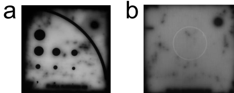
Figure 5.6 PL images of the P-doped poly-Si passivating contact samples (a) after Al metallization and (b) without Al metallization. The anneal setting for the samples presented here was 975 °C for 60 min. The PL settings were same to figure 5.3, *i.e.*, under 0.875 suns for 0.5 s.
