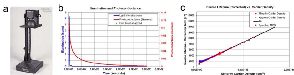
Figure 4.2 (a) A photo of Sinton WCT-120 lifetime tester [208]; (b) an example photoconduction decay curve; (c) an example inverse carrier lifetime curve.
