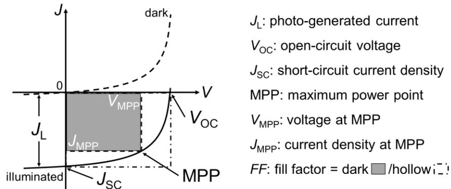
Figure 1.2 (left) Typical  $J$ - $V$  curves of a silicon solar cell under dark and illuminated situations. (right) The meanings of related items [13, 14].
