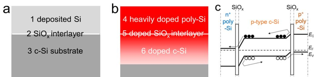
Figure 2.1 (a) A sketch of the precursor for a poly-Si passivating contact before the dopant diffusion process; (b) The basic structure of a poly-Si passivating contact; (c) the band diagram of n- and p-type poly-Si passivating contacts [90].
