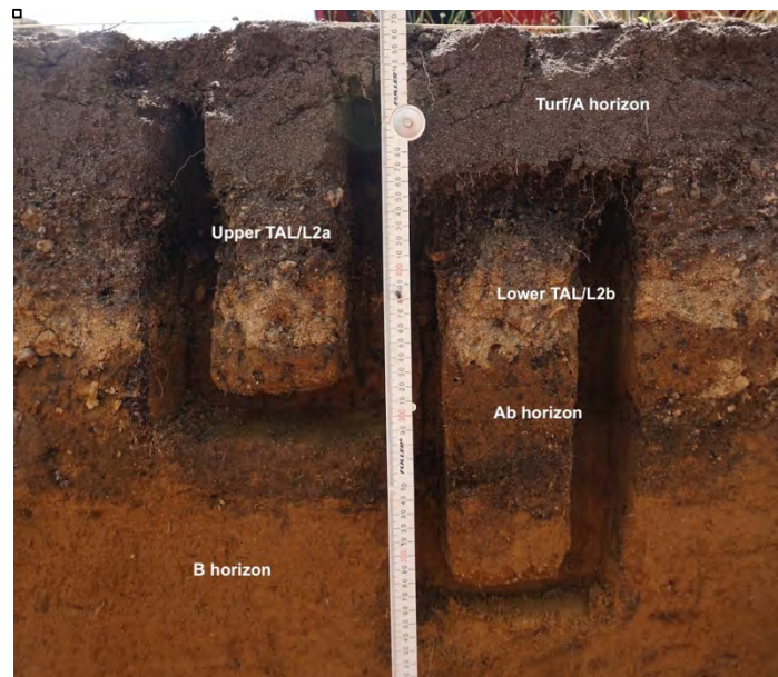
Figure 6.2: S15/424 samples LP1-II (left) and LP1-III (right) prior to the application of plaster bandages to encase the monoliths for micromorphological analysis.
