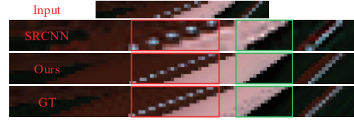
Fig. 7. Different types of continuity. From top to bottom, we show the input low-resolution EPI, super-resolved EPI from [51], ours and ground truth, respectively. Previous image super-resolution CNN copes well with “continuous continuity” (green boxes), failing for “discontinuous continuity” (red boxes).
