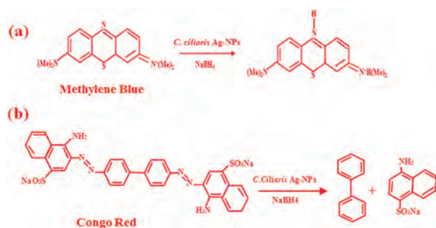
Fig. 5. Structure and reduced product of MB (a) and CR (b) by C. ciliaris Ag-NPs.
