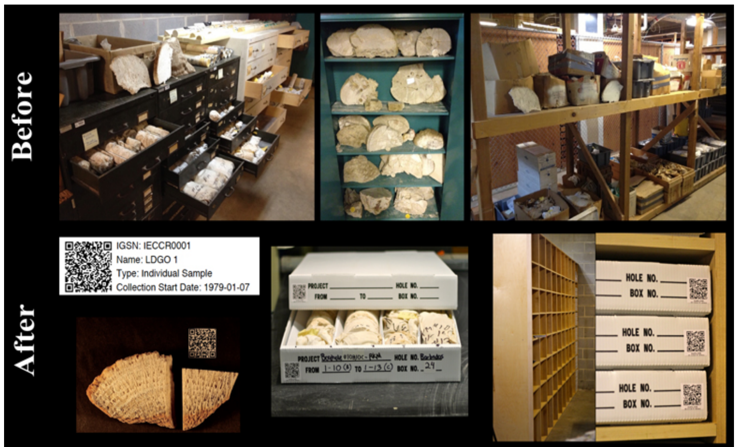
Fig. 1. Lamont-Doherty Coral Core Repository at Columbia University before and after organizing coral samples in boxes. Each sample was given an IGSN and Quick Response (QR) code for the
