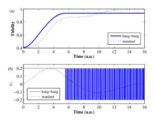
Fig. 1. The evolution curves of the fidelities with the target state (Fig. 1(a)) and the control fields (Fig. 1(b)) under the bang-bang Lyapunov control and the standard Lyapunov control, where the bang-bang Lyapunov control shows a high-frequency oscillation phenomenon.
