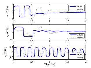
Fig. 5. The evolution curves of the three control fields under ABB Lyapunov control (40) (ABB II) and standard Lyapunov control (11) on a two-qubit superconducting system, in which the blue solid lines are the evolution curves of the ABB Lyapunov control, and the black dotted lines correspond to the standard Lyapunov control.
