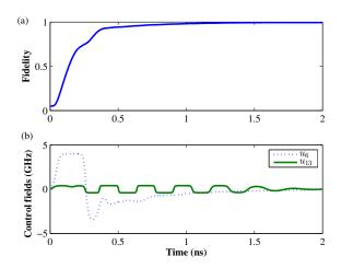
Fig. 6. (a) The evolution curves of the fidelity with the target state and (b) some control fields under ABB Lyapunov control (39) for an eight-qubit superconducting system, where only two ( $u_6$  and  $u_{13}$ ) of the fifteen control fields are plotted and the others are omitted.
