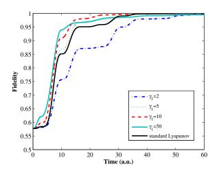
Fig. 3. The time evolution of the fidelities under standard Lyapunov control (11) and approximate bang-bang Lyapunov control (39) with different hardness parameter values.
