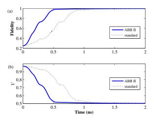
Fig. 4. The evolution curves of the fidelities (Fig. 4(a)) and the Lyapunov functions (Fig. 4(b)) under ABB Lyapunov control (40) (ABB II) and standard Lyapunov control (11) on a two-qubit superconducting system.
