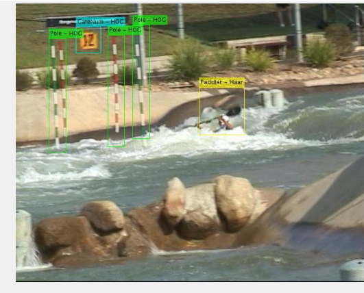
Figure 7: Gate poles and number detection using discriminative cascade classifier
