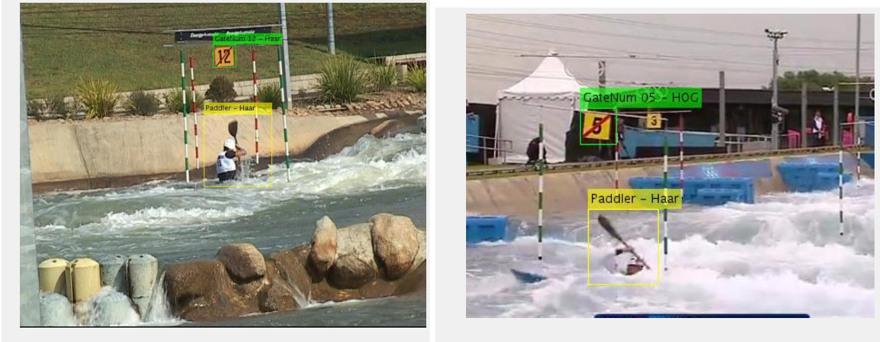
Figure 1: Our PPRDCF framework outputs location and scale of the slalom paddler, and the location and order of the gates.
