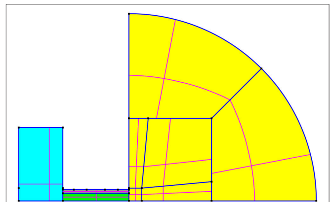
FIGURE 2 | Two dimensional cross section of the axisymmetric top half of the PR mesh, with the four regions: plenum (cyan), discharge volume (green), downstream (yellow), and cavity wall (gray). Blue lines denote the interfaces between adjacent regions or subregions. The magenta lines show the position of the median cell in each region or subregion. The inlet is defined to be the cylindrical surface of revolution formed by the top edge of the plenum, and the outlet is the hemispherical surface on the far right of the downstream region. The front plenum wall is defined to be the left internal face of the plenum region, while the rear plenum wall is the right internal face of the plenum region surrounding the entrance to the discharge volume region.
