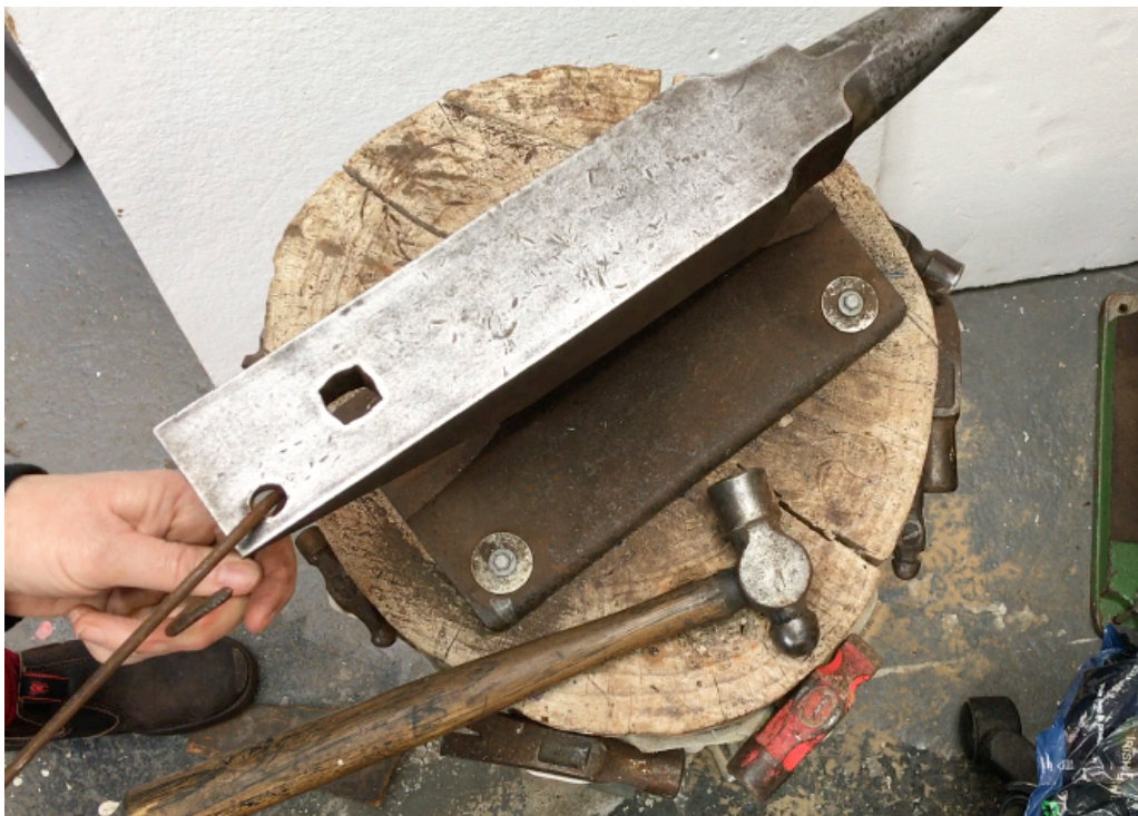
Figure 27. Bending the steel in the top of the anvil for The Honeymoon Day 1 .
